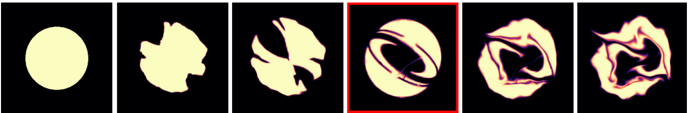
Fig. 12. Inverse fluid control by optimizing the initial velocity field to match a SIGGRAPH logo target. Frames progress left to right; the red rectangle indicates the target frame.
